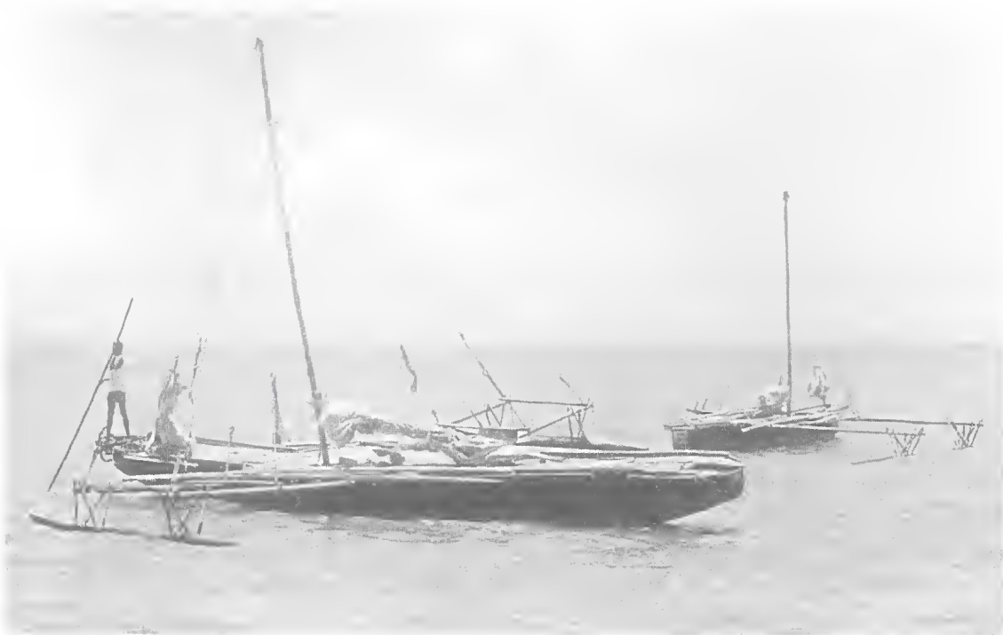
FIG. 57. Double outrigger, single masted pupto canoe 'Delasa' and single outrigger, single masted tatau canoe at Daru.
